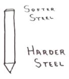
being split. If the end of the hammer or chisel was hard, and the hammer was hard, it could end up with either the hammer or chisel being damaged. So, as a compromise, chisels are designed to "wear out" by mushrooming and thus protecting the expensive hammer from damage.
