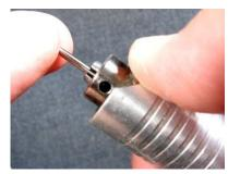
For closing the jaws around a smaller shaft, there's a neat trick. Hold the new bit in the center of the open jaws of the chuck, put your thumb lightly onto the outer toothed collar of the chuck, and gently start up the Foredom. As the chuck turns, it will naturally tighten the jaws around the bur shaft or the drill bit. Then all you have to do is a final tightening with the key.
