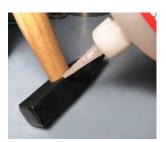
a hammer head. The traditional way to tighten a loose hammer head is a bit of work with wedges, but if the head is basically secure, there's a fast and easy way to tighten a loose head for about 50 cents - superglue.
