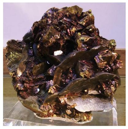
Chalcopyrite's primary commercial use is as an ore for copper. It has been the most important copper ore for thousands of years. It can be roasted in with silica sand in open air or an oxygen rich atmosphere to produce copper, sulfur oxide, and iron silicate. The chemical formula for the roasting is:
