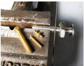
Whenever you have to cut a threaded bolt shorter, it's often difficult to get the nut to thread back onto it. And the smaller the bolt, the more difficult it is to restore any distorted
