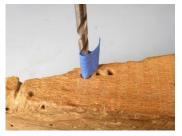
Sometimes you need to drill a number of holes all to the same depth. One quick and easy way to do this is to wind some tape around the drill bit so that the tape just touches the part's surface when the
