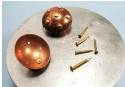
For best results, select a drill that gives you a hole with a close fit to the rivet. Trim the rivet to leave a little less
